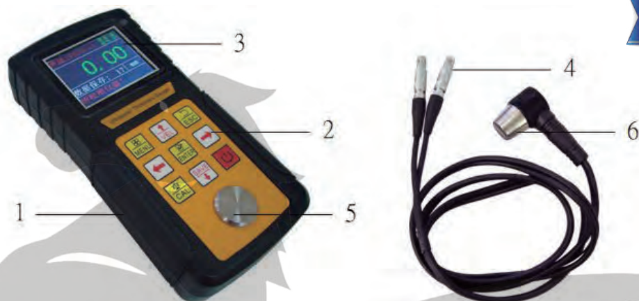
1.Shell 2.Keyboard 3.Monitor 4.Transmit & receive socket 5.Thickness calibration block 6.Ultrasonic probe
