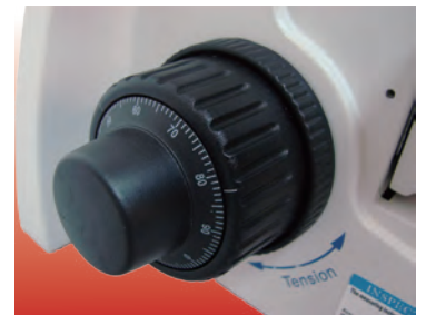
Coarse & fine adjustment focus knob.
