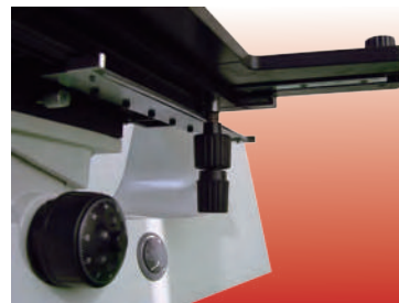
X, Y-axis slide guide
