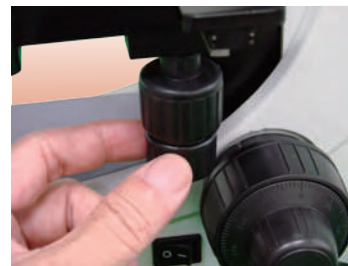
X, Y-axis slide guide
