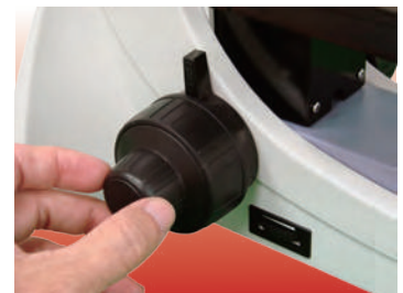
Coarse & fine adjustment knob.
