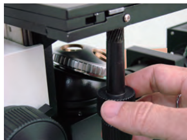
X, Y-axis slide guide
