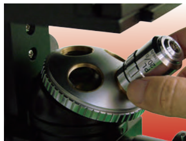
4 convertible objective lens units
