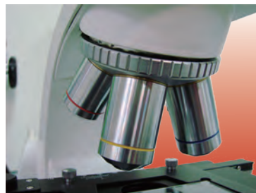
4 convertible objective lens units
