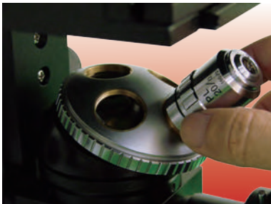
4 convertible objective lens units
