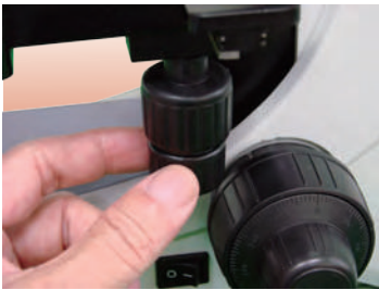
X, Y-axis slide guide
