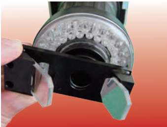
3D Stereo reflecting mirror
