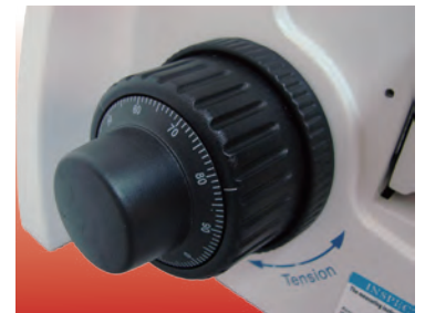
Coarse & fine adjustment focus knob.
