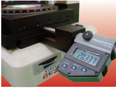
X-Y measuring table and micrometer head
