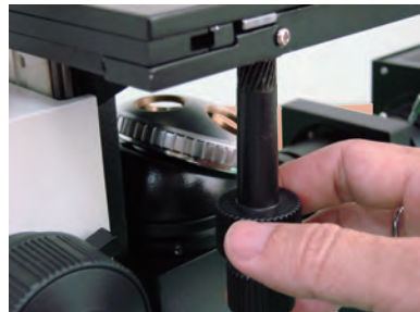
X, Y-axis slide guide
