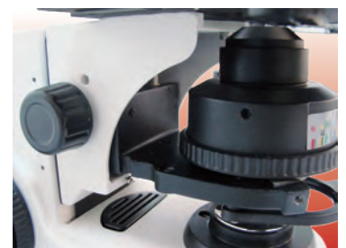
Up & down adjustment knob for condenser
