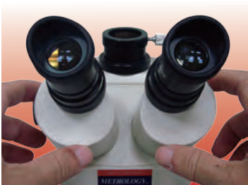
Dual eyepiece & CCD port
