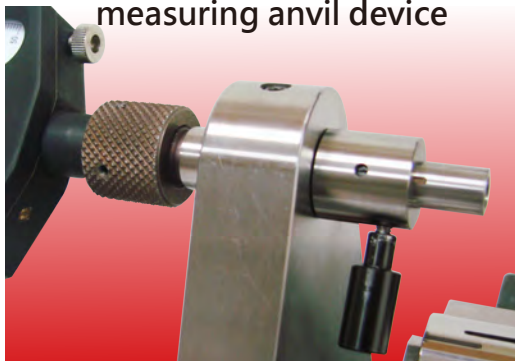
UMC-ITD Anvil inside diameter \Phi 5\text{mm} indicator optional
