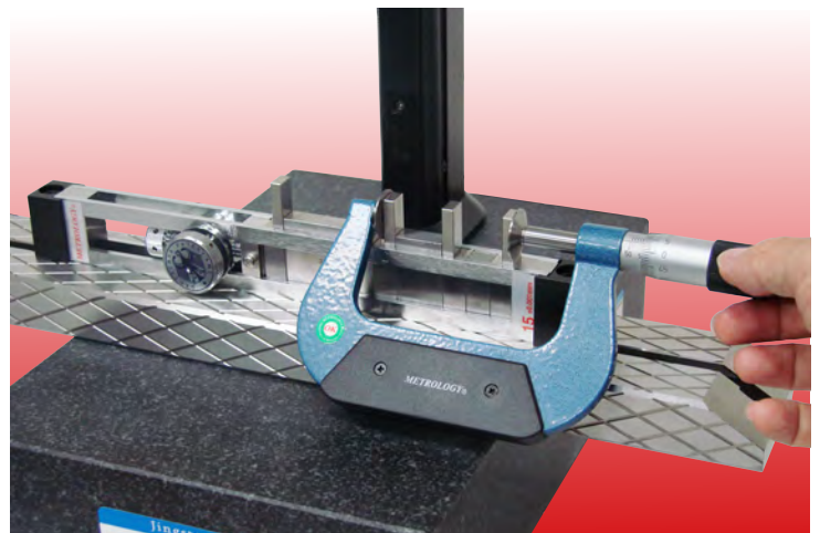
Calibrating inside and outside micrometers (Calibration point: 5mm per step)
