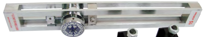
UMC-GH1S Gauge Block Hold Standard and fixture set Calibration range 0-200mm
