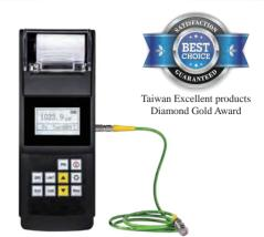
In addition to the features of the general Coating Thickness Gauge, this instrument is also equipped with a printer device that can print test result data and can be connected to a computer by installing general software for data output, storage, report printing, etc.
