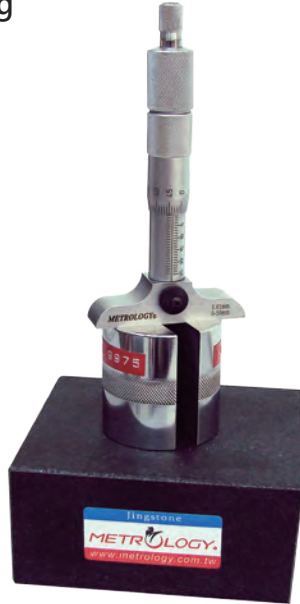
Depth micrometer calibration & zero setting
